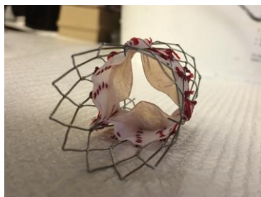
Figure 6 : An aortic valve prototype using flat sheet Bacterial cellulose cut and sutured on to a stent 21
